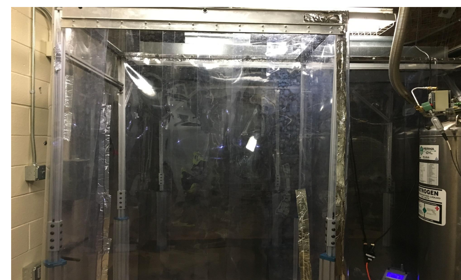
Figure 4. Softwall Cleanroom on the 4850L of SURF.
