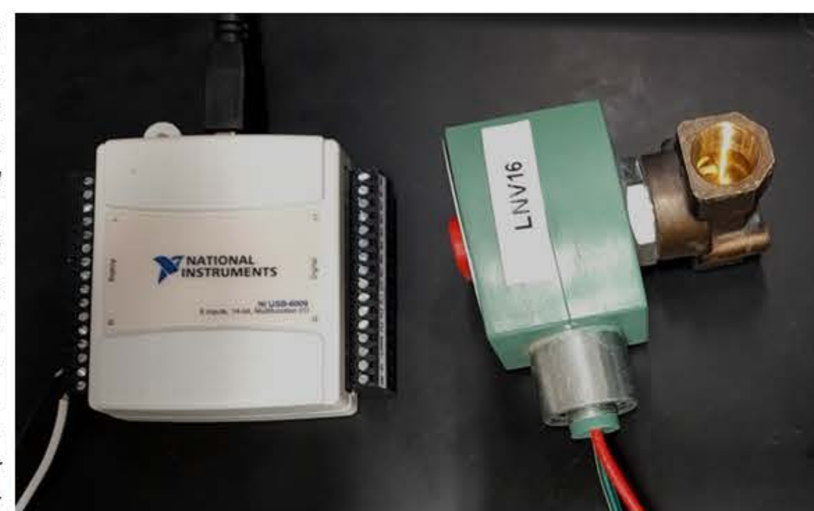
FIG. 4. The NI USB-6009 DAQ (left) and ASCO Red Hat 2 solenoid valve (right). The DAQ was used to output an on/off (0V or 5V) signal to the valve, though a COM-13015 solid state relay was wired between the two in order to swap the DC signal to AC. Another valve of the same kind was wired into the system to be used for precooling, but the code for this was not completed. Adding the precooling system could be the next step in further work on the project.
