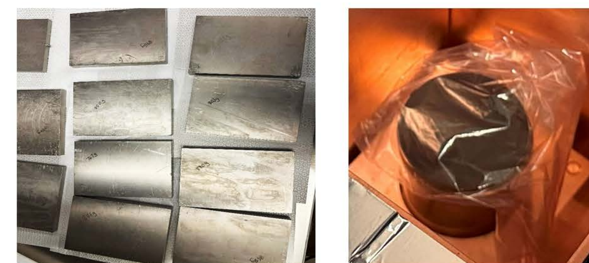
FIG. 6. Titanium samples counted at BHUC (left) and dried ink from 48 sharpies emptied into a petri dish placed in Mordred (right). The petri dish was covered with a plastic bag to ensure that Mordred would remain clean.
