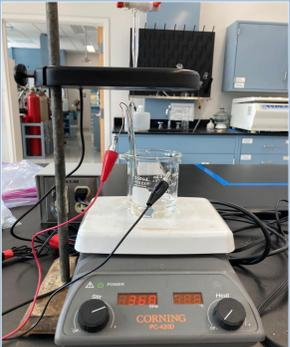
**Figure 2:** Potentiometric Titration for water sample Cl<sup>-</sup> ion concentration
