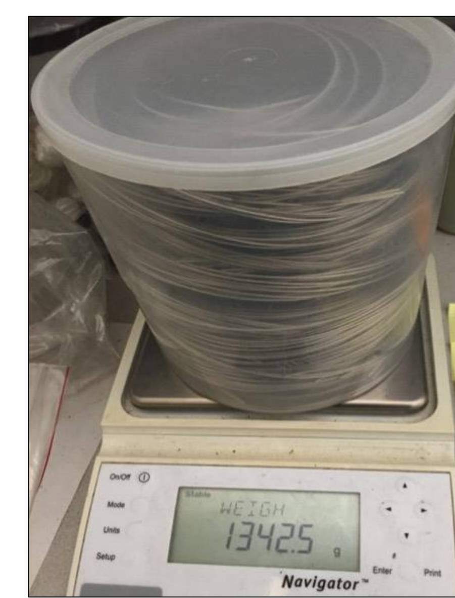
Figure 2 – (left) Detector crystal and aluminum plate sample in a crystal annulus geometry. (right) A sample of titanium wire prepared in a full geometry. In both examples a standard sized "Marinelli beaker" is used to control the counting geometry.
