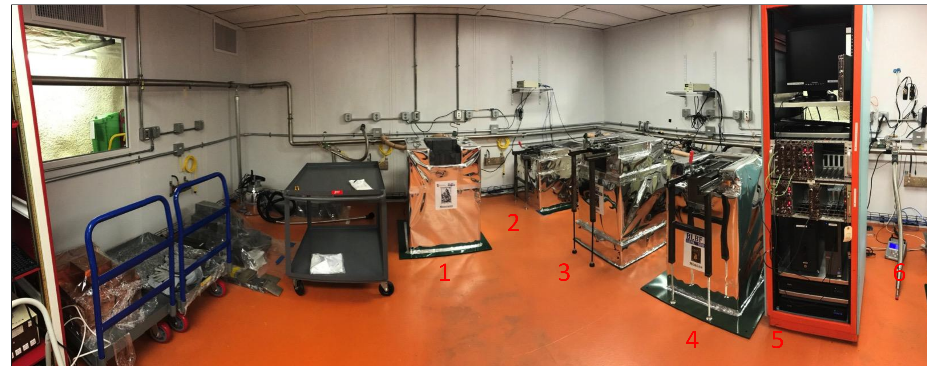
Figure 1 – BHUC cleanroom. Shown: Mordred (1), SOLO (2), Maeve (3), Morgan (4), the electronics responsible for networking and data acquisition (5), and the particulate counter (6).
