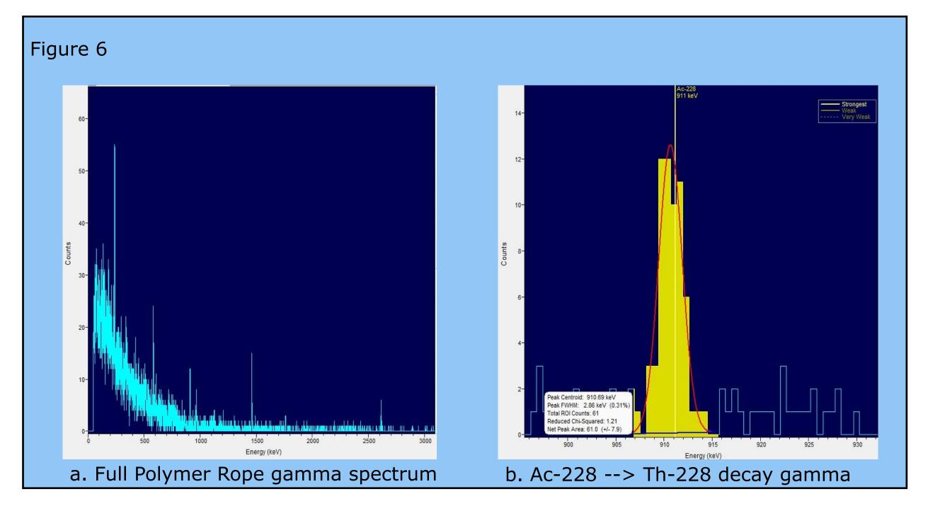
The total energy of the peak is given by the area beneath the curve, figure 6b, which is used in the following equation to find the nuclides concentration C:
