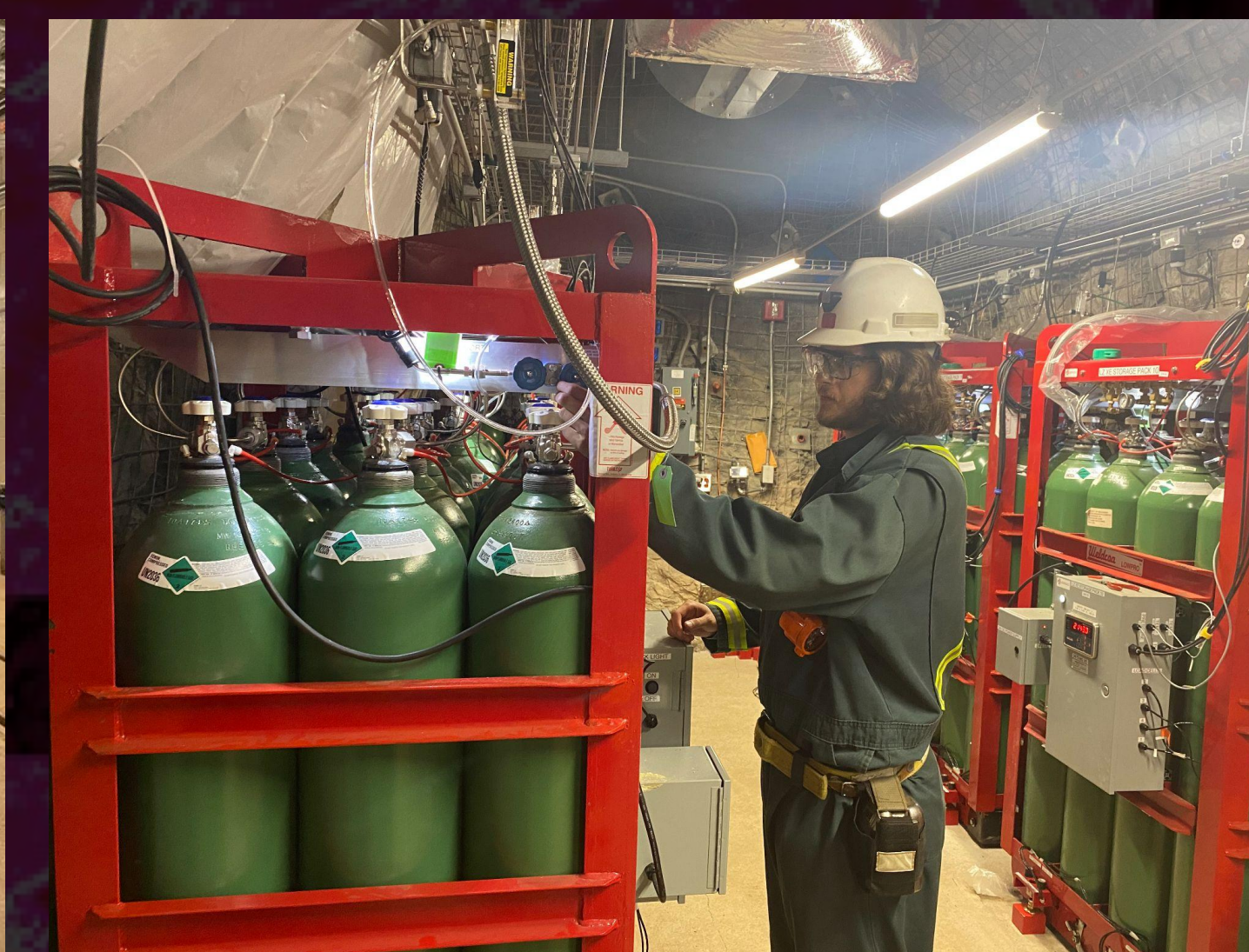
Jax Wysong in the Xenon Room. As the name implies, this is where all the xenon gas is staged that will eventually be moved into the TPC and condensed into liquid form. LZ uses about 10% of the world's annual production of xenon!
