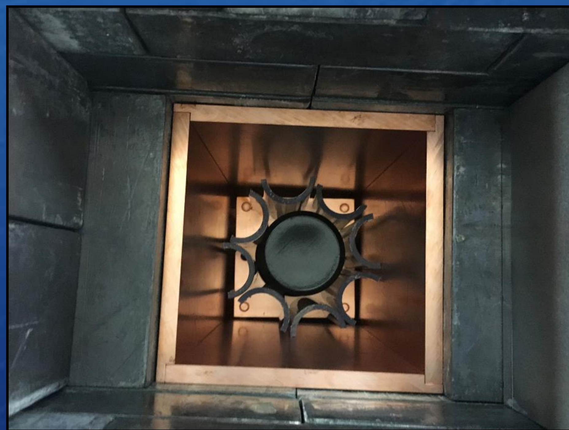
Figure 2. Pieces of pipe around a HPGe detector.
